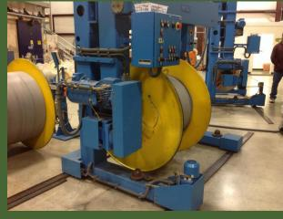
properties of the cable. Then it is re-wound onto another cable reel. Cross-linking enhances the thermal, chemical and electrical stability of Thermon's low-temperature self-regulating heater cables. All end products produced at Thermon's San Marcos plant must go through ECLF uncoiler and re-coiler stations for
