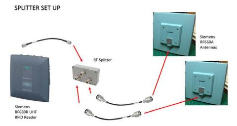
Figure 3: Showing how using an RF Splitter can allow for additional antennas to be added to a port.
